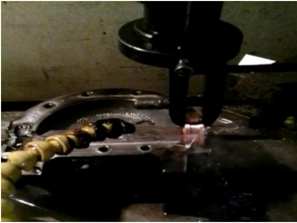
Fig. 5: Set up for EDM operation for spherical chamber
